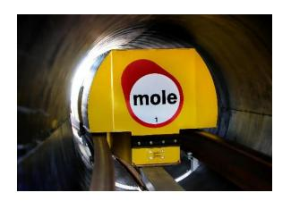
Bulk (mining)cargo 1.3m dia - 5 Tonne
