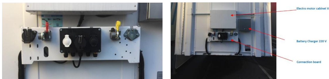
Figure 30: Connector on trailer to charge battery
