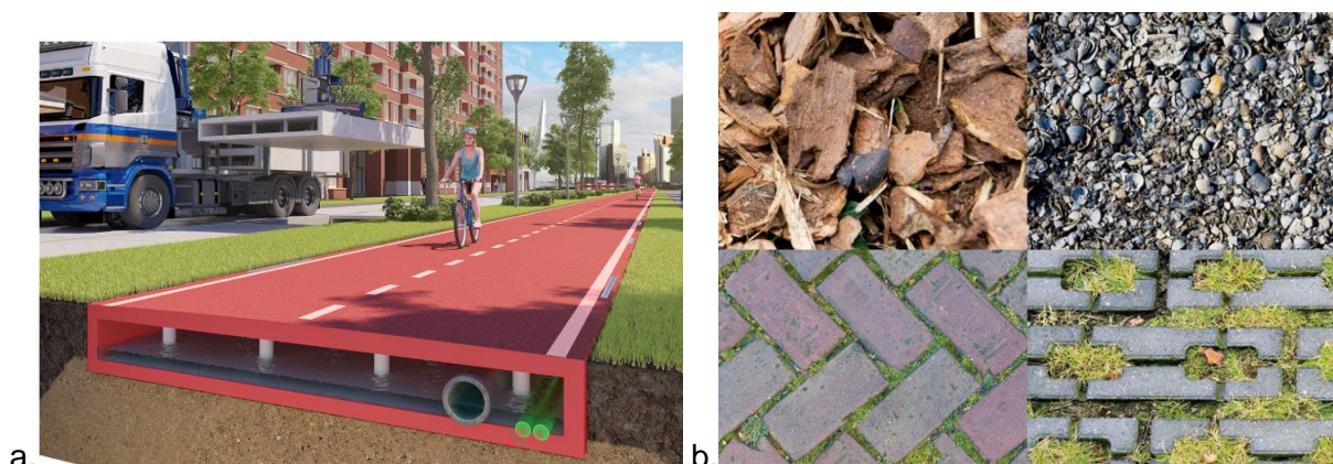
Figure 5: Materials for road construction a) Plastic-road, b) porous paving materials
