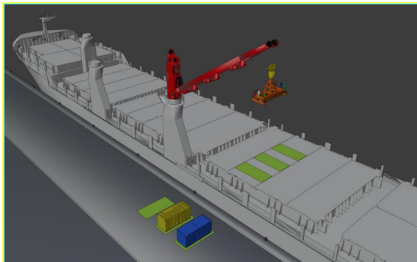
Figure 2. Innovative feeder vessel equipped with Robotic Container Handling System
