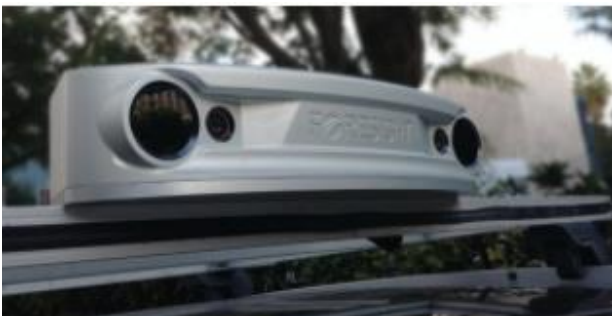
Figure 4: QuadSight vision system by Foresight 2
